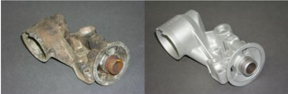
Gambar. 10.1 hasil sand blasting
